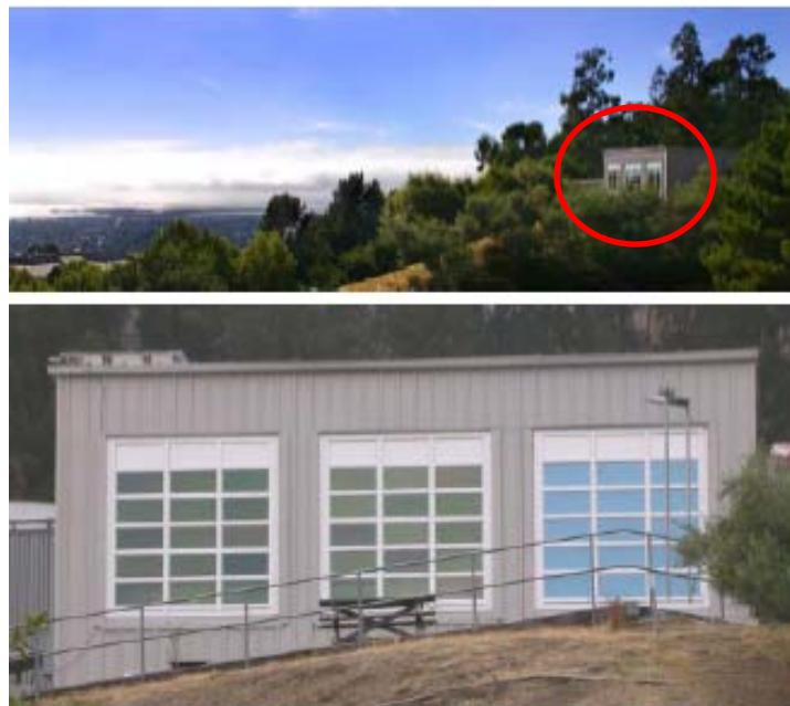
Figure B-3. LBNL Window Test Bed Facility (upper photo). South elevation of EC facades (lower photo) (Lee, et al., 2006).
